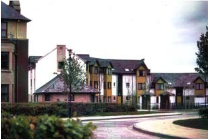
The form of the buildings became ever more related to passive solar gain and a preference for large south and small north facing windows. Phase 7 formed a sun-scoop using a permaculture garden design. The extent of landscaping is rich and varied, and allows for larger areas of soft and porous surfacing. The next phase under development contains low allergy materials and finishes. The ventilation will use dynamic insulation.
